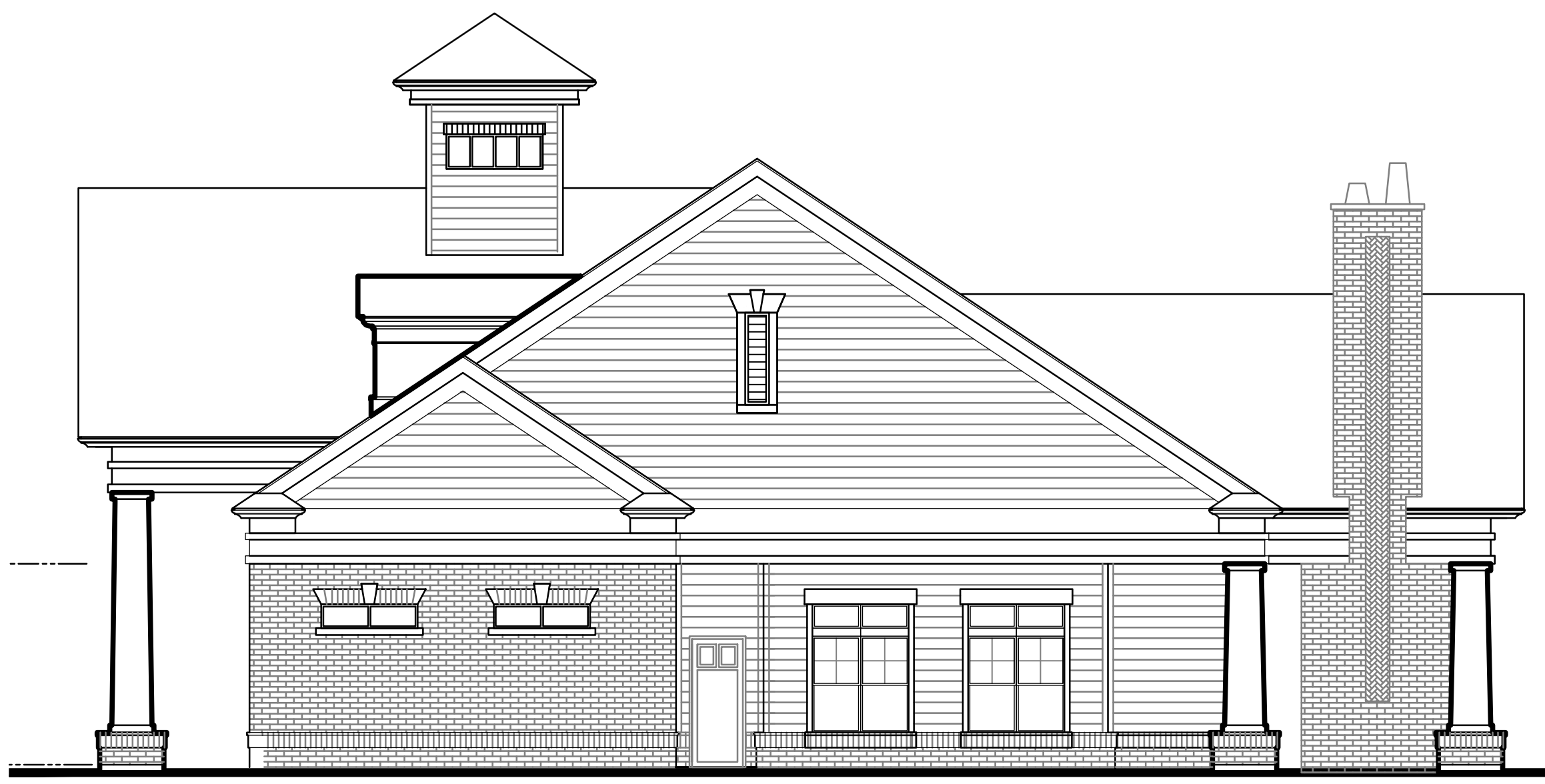
2 CLUBHOUSE/LEASING CENTER RIGHT SIDE ELEVATION 1/8" = 1'-0"
