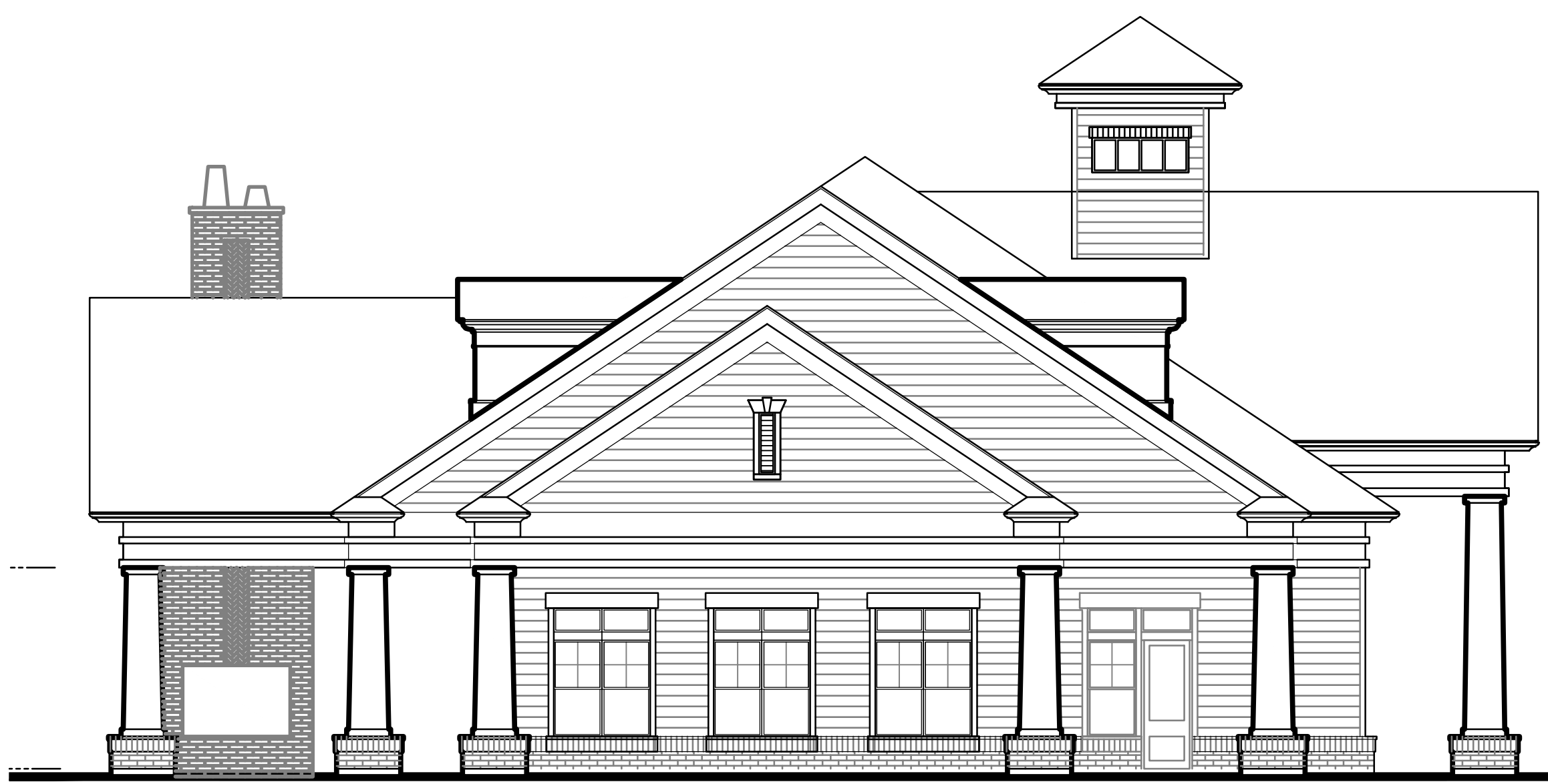
4 CLUBHOUSE/LEASING CENTER LEFT SIDE ELEVATION 1/8" = 1'-0"
